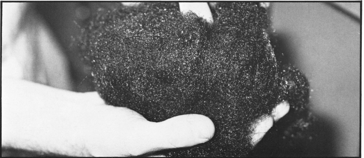
The waste acetate that is cut out of the groove is called "chip". By means of a vacuum system, it is sucked into a receptacle for disposal.
