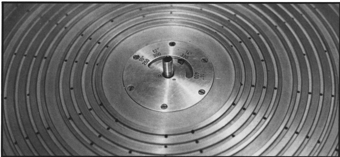
Close-up of the turntable of a Neumann Lathe, showing disc size selector and vacuum holes for disc hold-down.
