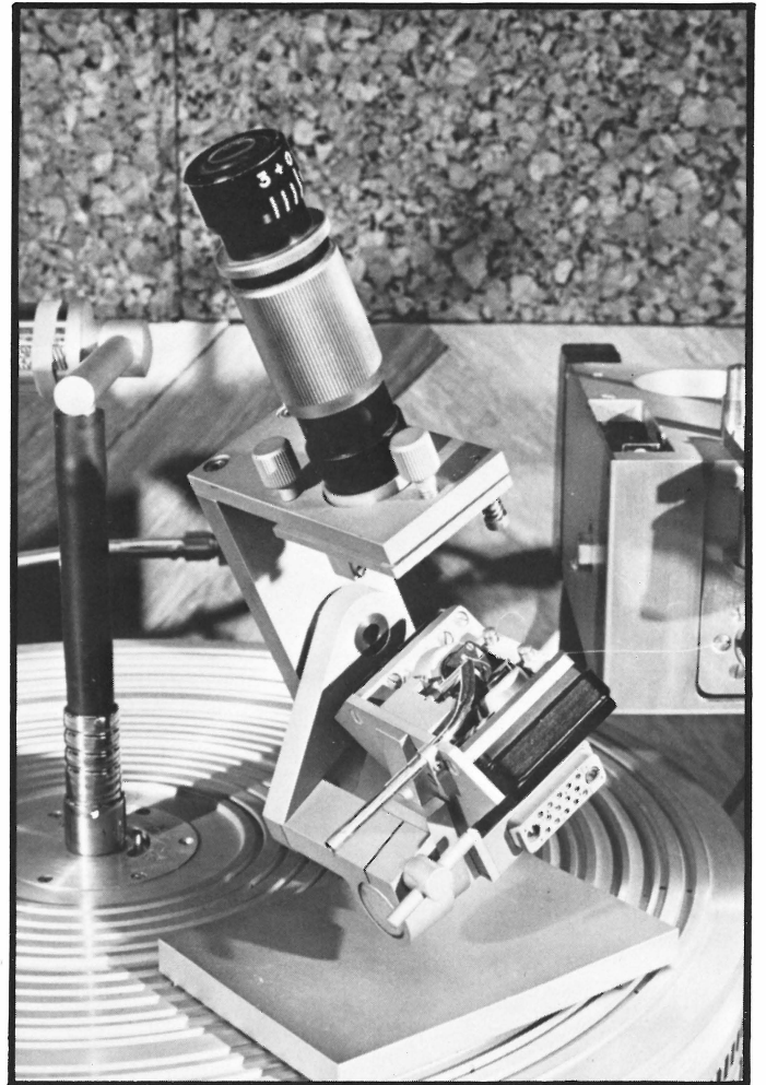
A second, smaller microscope is used to mount the cutting stylus in the cutterhead.
