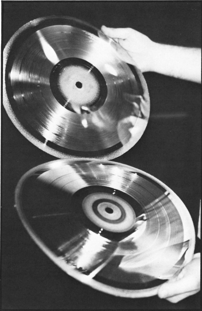
The final stamper is separated from the metal mother.
