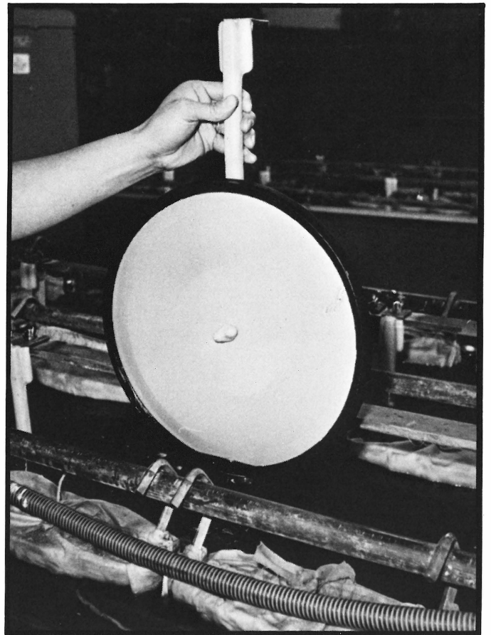
Once coated with nickel at the proper thickness, the acetate is removed from solution.
