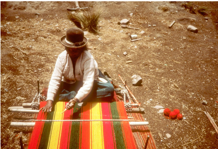
Figure 1.10. Aymara woman in 1988, Lakaya village, Lake Titicaca, Bolivia. She is working on a horizontal loom using a pick made from a llama legbone.
